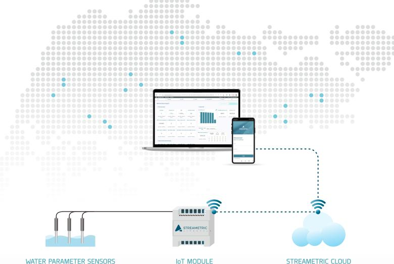
Installed inside the pump room, the sensor probes detect pH, Free chlorine, Temperature and ORP levels of your Aquatic Facilities.
